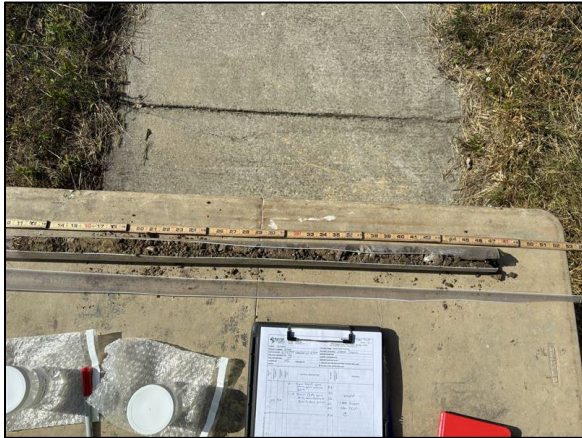
Photo 13: View of soil recovery at the time of TCLP sampling
