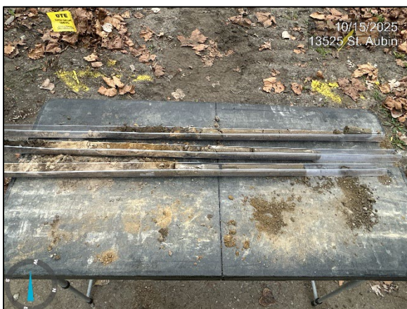
Photo 5: Viewing soil recovery from 13525 SB-1, SB-2, and SB-3
