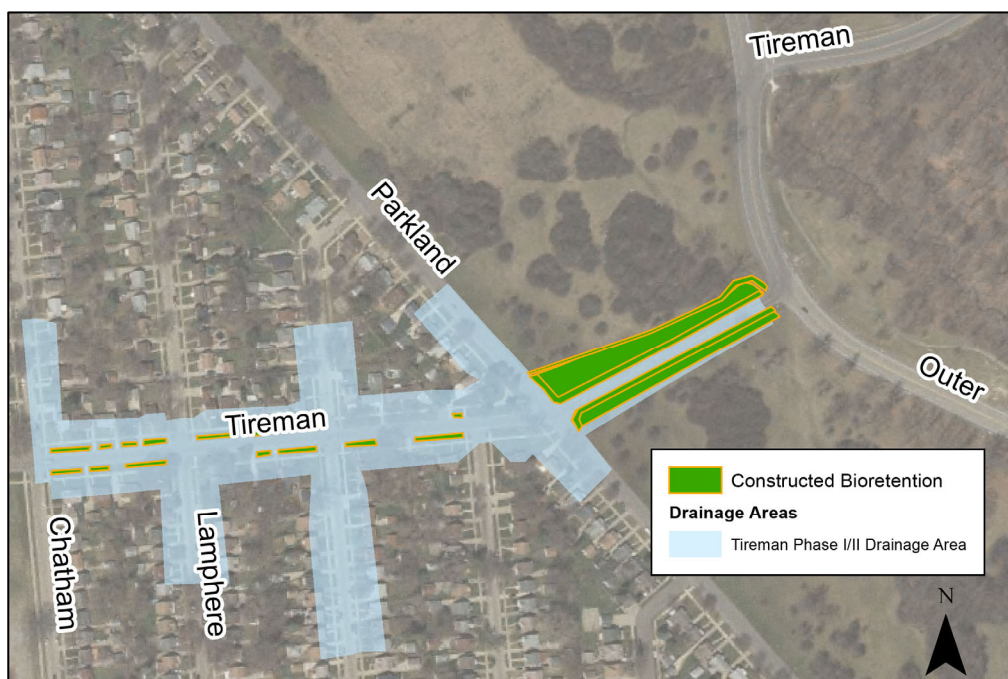
Figure 10: Tireman Bioswales – Drainage Areas
