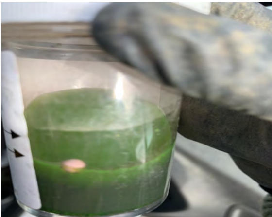
Side view of negative dye test at soil boring location SB-14. Photo taken by Rabia Azam on 1/14/22
