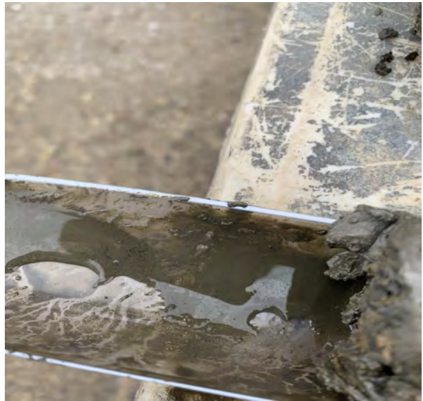
Close up of sheen at 15 ft bgl in soil boring SB-11. Photo taken by Rabia Azam on 1/12/22
