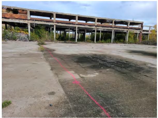
Facing east, viewing marked GPR linear anomalies. Photo taken by Patrick Howe on 10/22/21.
