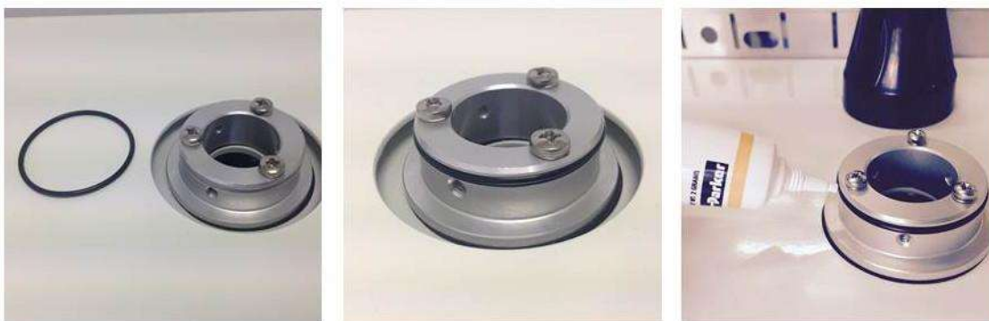
Figure 2-2 Add the O-ring and a small amount of lubricant.
