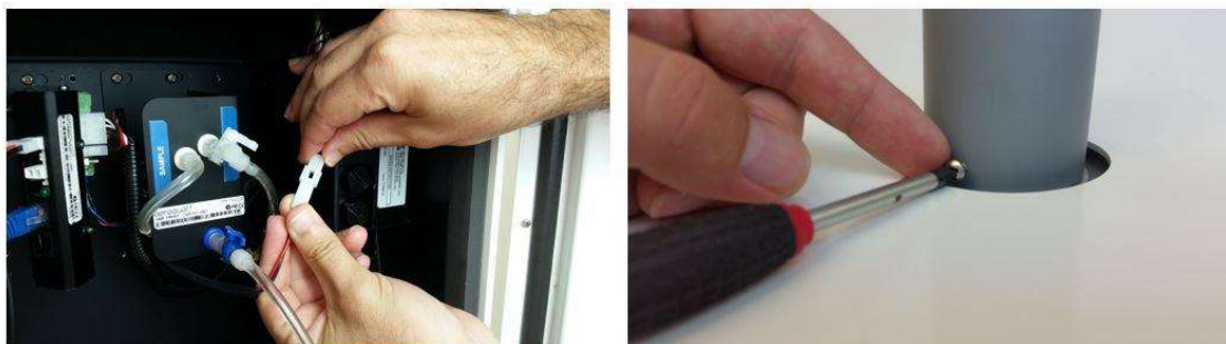
Figure 2-6 During field installation, secure the PM inlet using the retaining screws and plug in the heater
