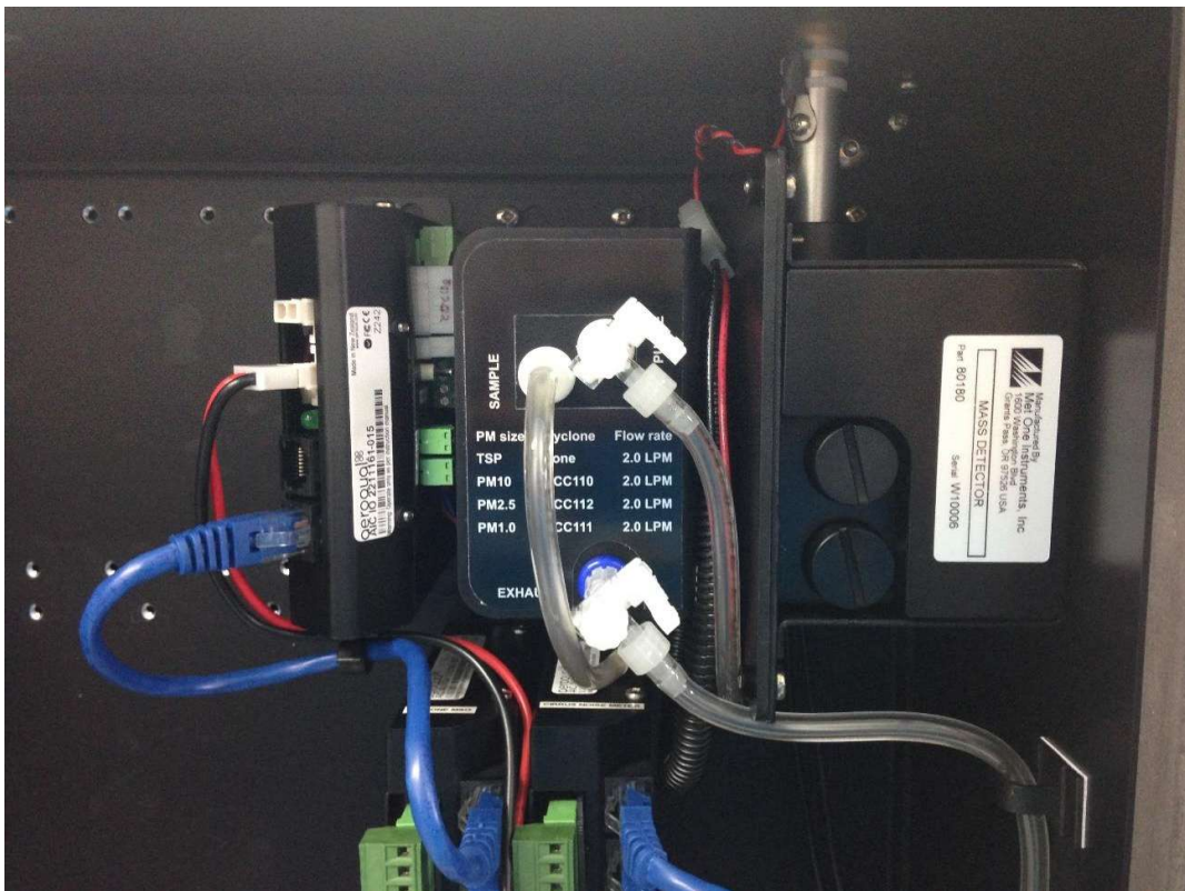
Figure 12-4 The Particle Monitor uses three modules: a) the optical engine on the far right, b) the pump module in the middle, c) the I/O module on the left
