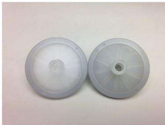
Figure 6-6 The particle filter on the gas inlet can be easily replaced, it should be replaced when it gets dirty as shown in the image on the right (a new filter is shown on the left, dirty filter on the right).
