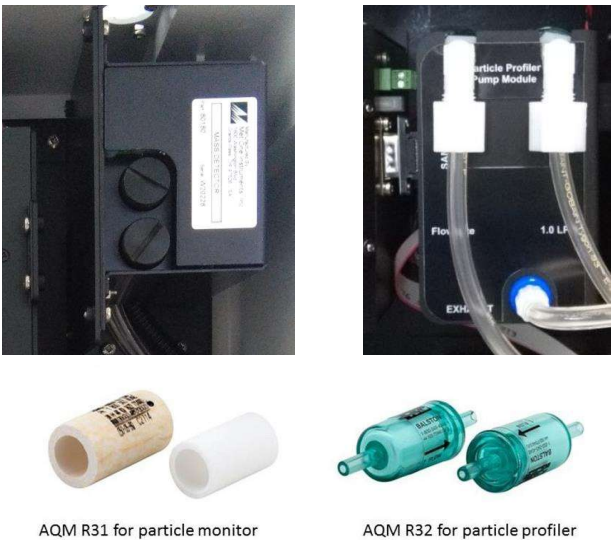
Figure 6-9 The Particle Monitor (shown on the left) requires AQS R31 and the Particle Profiler (shown on the right) requires AQS R32
