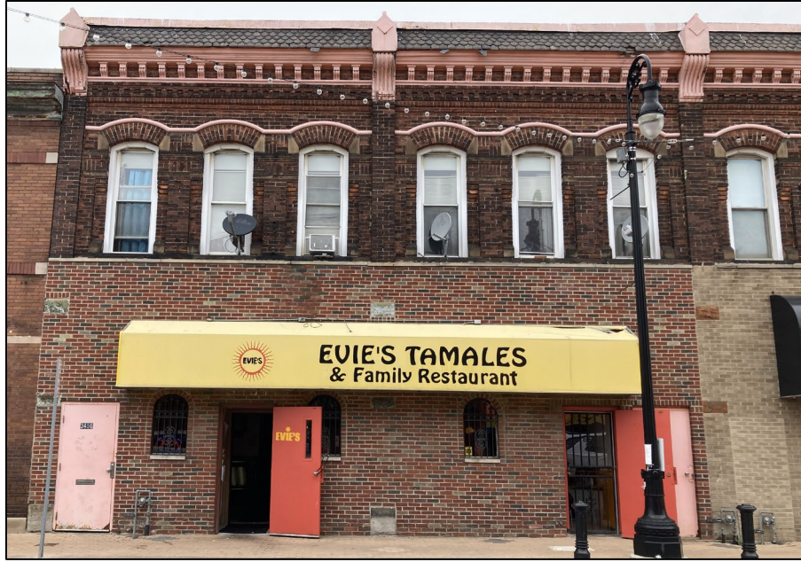
Figure 55. Example of infill of first-floor windows and the covering of an original storefront to a commercial building in a proposed district. (Kraemer Design Group, 2023)
