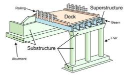
Figure 34 - Diagram of Bridge Elements
