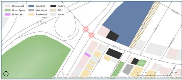
The intersection of Fort Street and Schaefer Highway is surrounded by areas predominantly commercial and industrial. The pavement rating is poor for Schaefer Highway and fair for Fort Street, based on PASER ratings. The Issues highlighted in this area focused on the damaged road conditions due to truck usage. The recommended improvements for this intersection are as follows:
