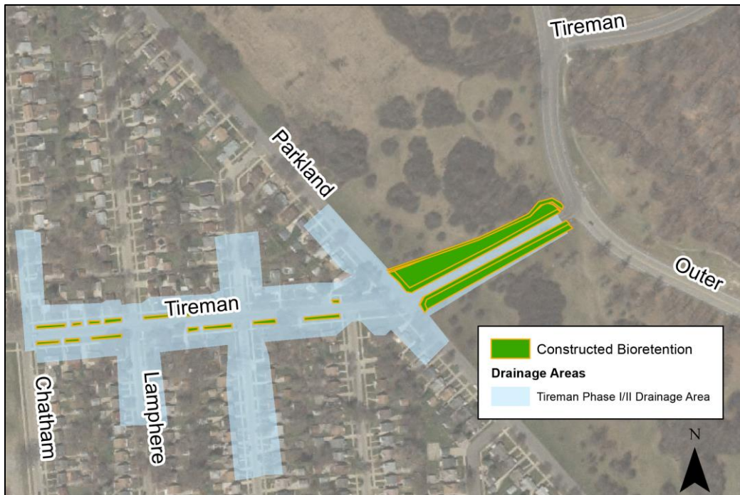
Figure 11 Tireman Bioswales – Drainage Areas
