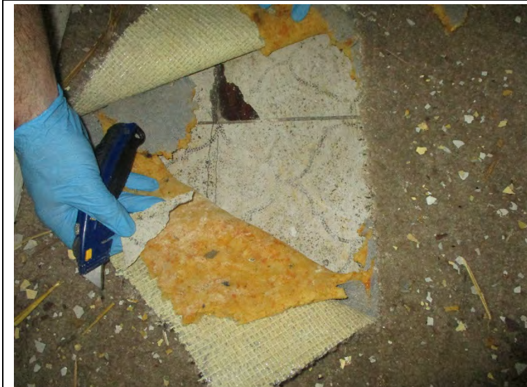
Photo 5. View of asbestos-containing Cream/Brown floor tile in the hallway of 2251 Sheridan, 2 nd floor
