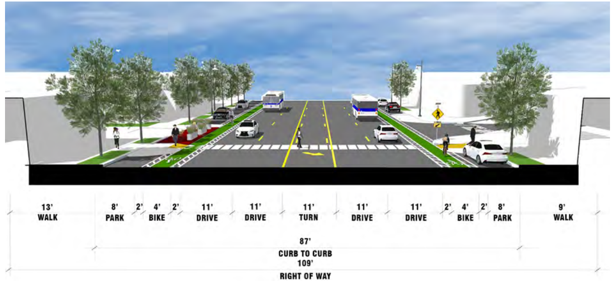
Proposed Street Section on Grand River Avenue Between McNichols Road and Cooley Street
