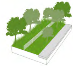
Step 1: Interim repairs to perimeter fence
