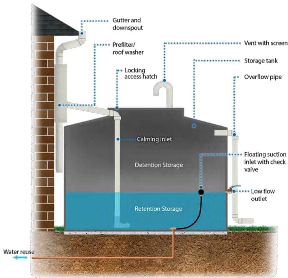
**Figure 11-8 Cistern for detention and retention storage**
