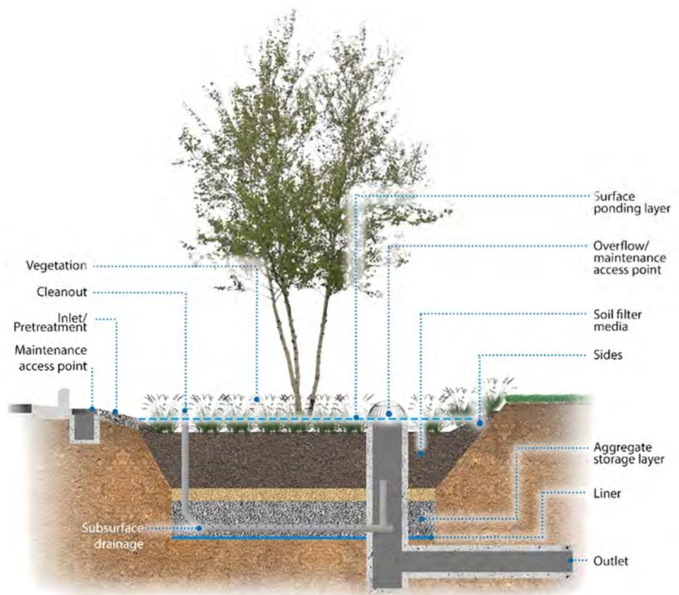
**Figure 8-1 Components of a typical bioretention practice**
