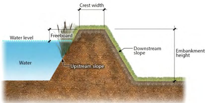
**Figure 7-7 Embankment Illustration**
