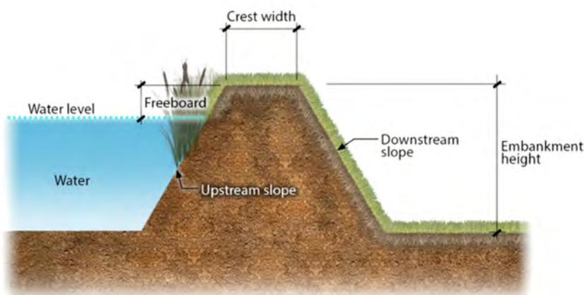
**Figure 7-7 Embankment Illustration**
