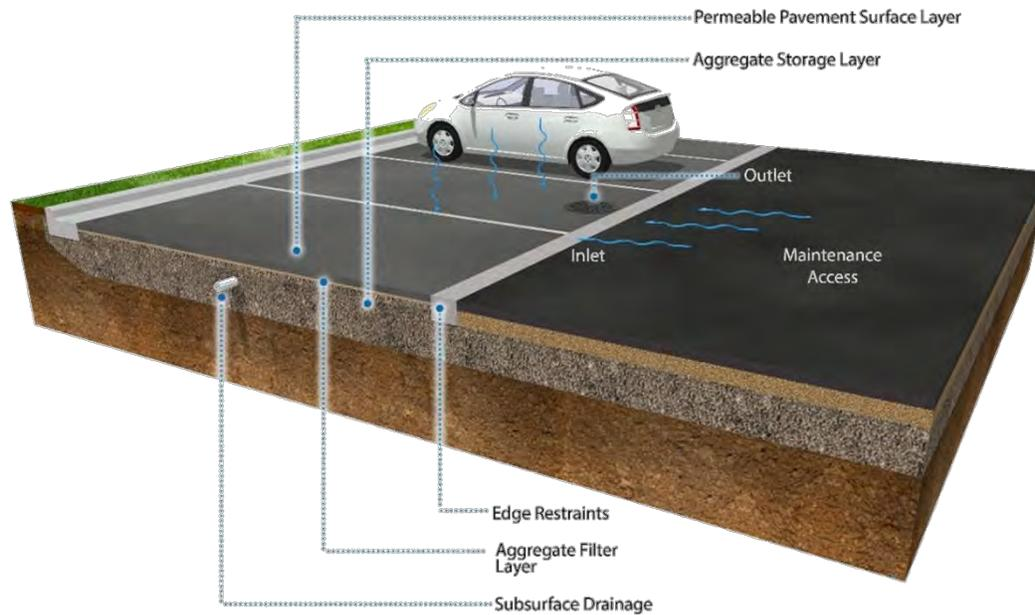
**Figure 10-2 Components of a typical permeable pavement practice**
