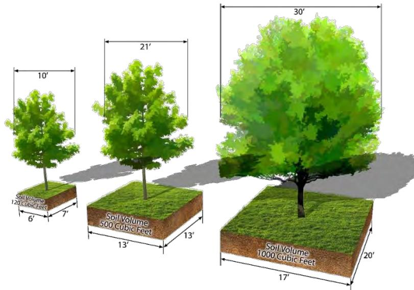
**Figure 15-13 Typical recommended soil volumes by canopy size**
