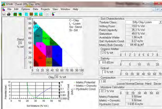
Another useful tool is the USDA Soil-Plant-Atmosphere-Water (SPAW) Field & Pond Hydrology model. Contained within the SPAW model is a Soil Water Characteristics tool. This tool provides estimations for the saturation porosity, field capacity, saturated hydraulic conductivity and other soil characteristics based on a soils sand, clay and organic matter content. The SPAW model is available at:
