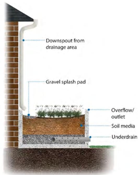
*Figure 8-30 Bioretention cell with a sealed drainage profile*
