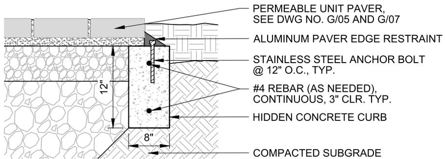
**METAL EDGE RESTRAINT ON HIDDEN CONCRETE CURB
