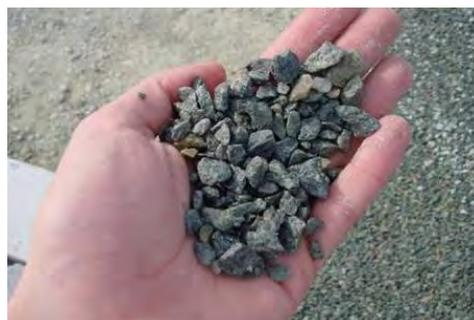
MDOT standard aggregates, Table 6-5, typically need to be washed thoroughly prior to using in a GSI practice. Loss by wash, i.e. passing the No. 200 sieve, should be less than 0.5%.
