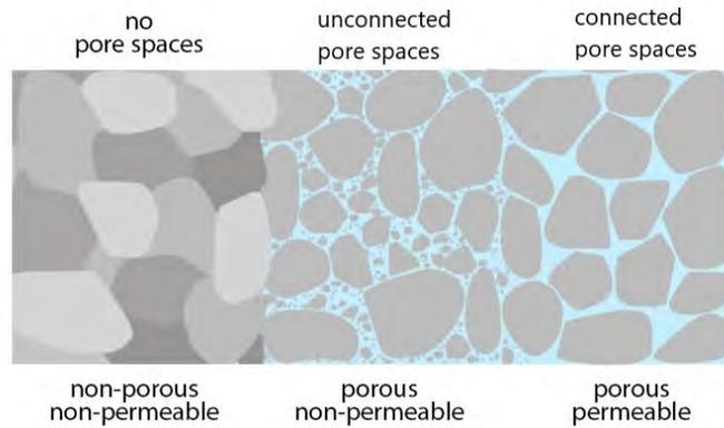
**Figure 6-2 Porous vs Permeable Illustration**
