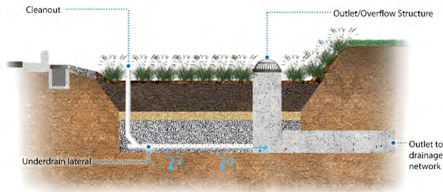
**Figure 8-27 Bioretention cell with a conventional drainage profile**
