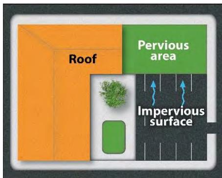
*Figure 3-5 Disconnected impervious surface draining to lawn*
