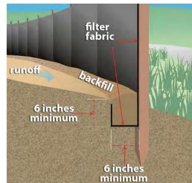
**Figure 3-14 Silt fence**
