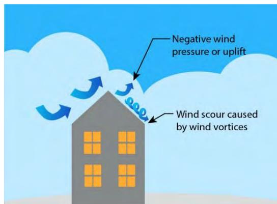
*Figure 12-9 Effects of wind on roofs*
