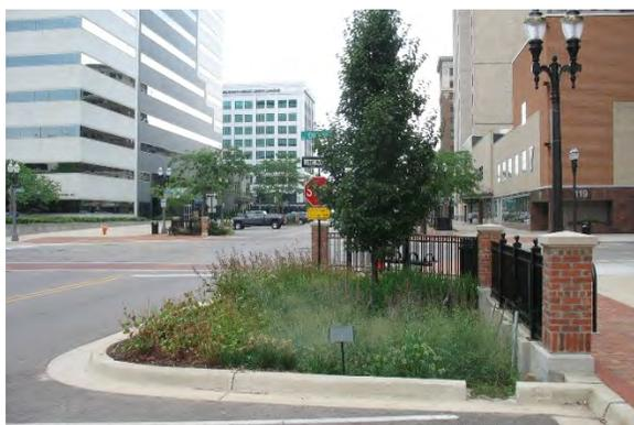
**Figure 8-10** *CBD Curb Extension Bioretention*
