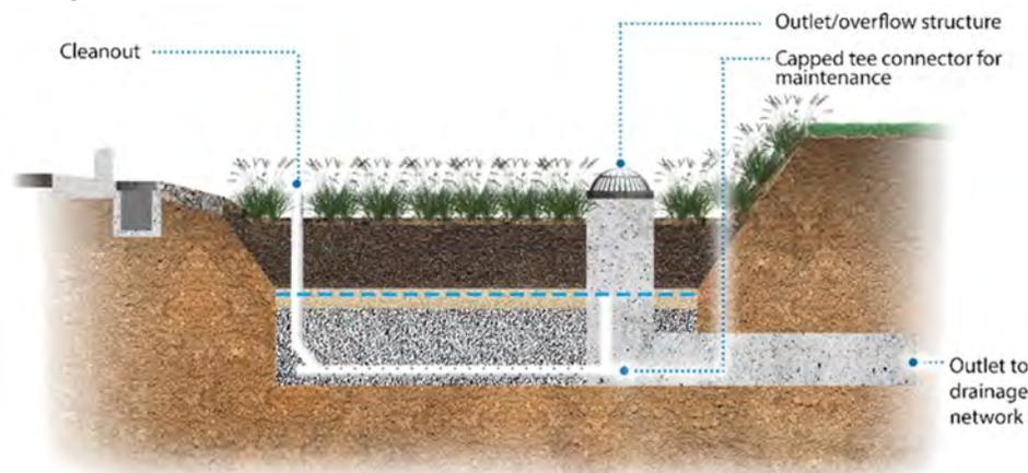
**Figure 8-28 Bioretention cell with a saturated zone drainage profile**
