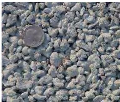
**Figure 10-4 Example of Pervious Concrete**
