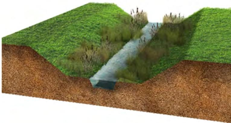
*Figure 5-1 Two-stage channel*
