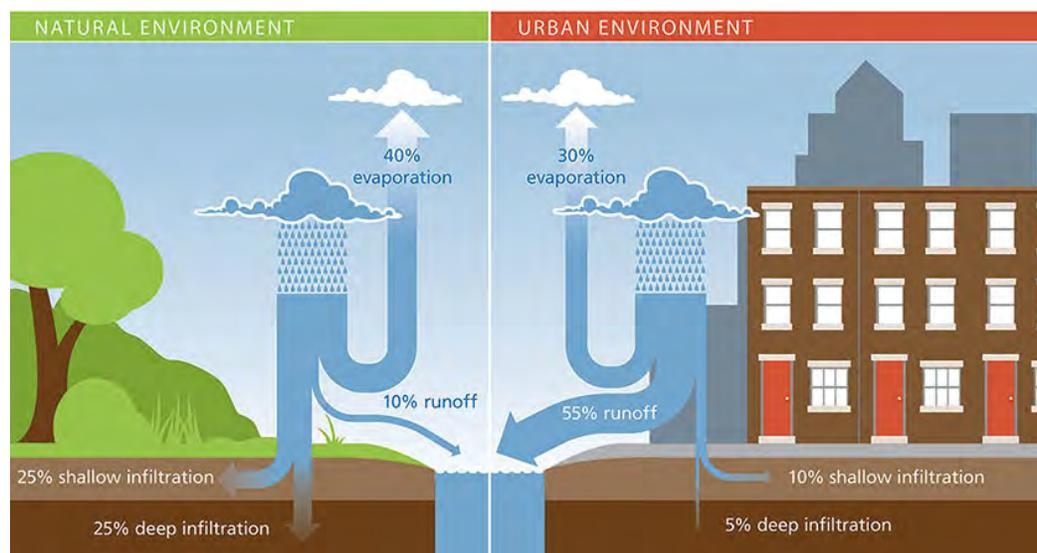
**Figure 1-1 Impacts of urbanization on the hydrologic cycle**
