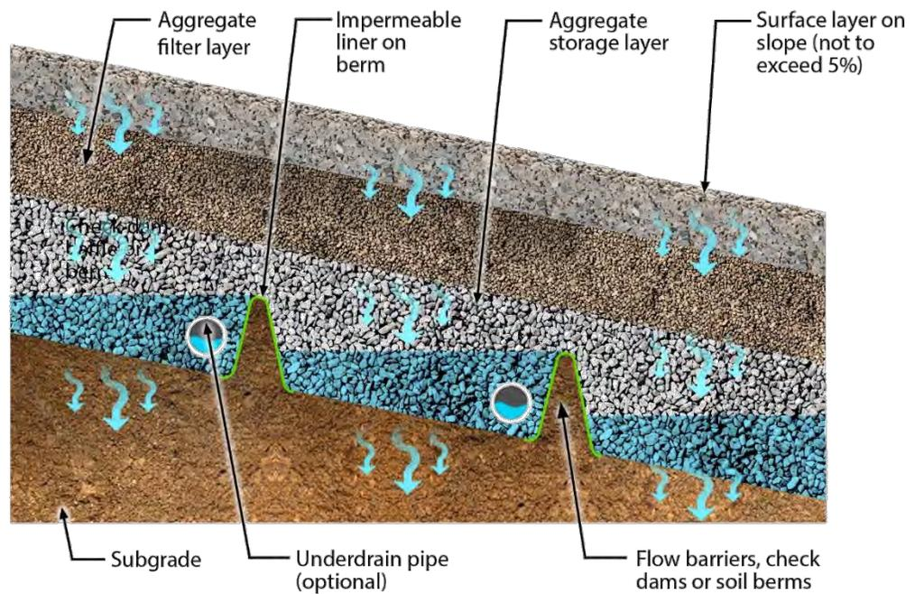
Figure 10-21 Steep slope drainage profile with sloping subgrade
