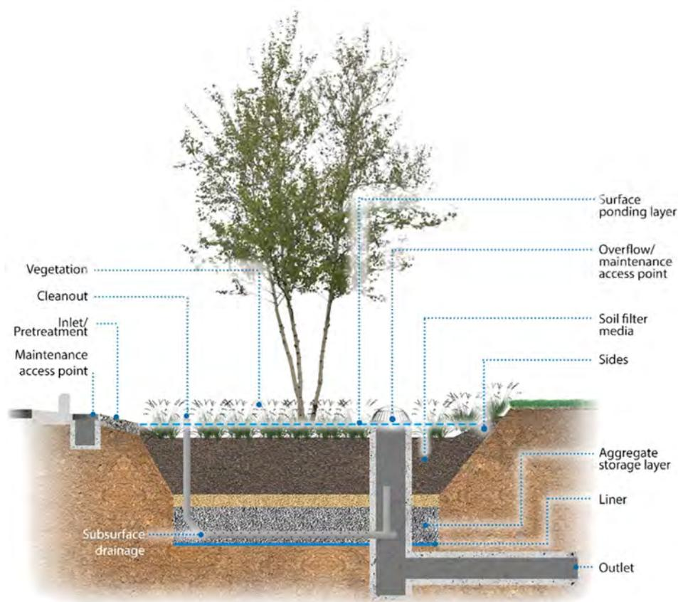
**Figure 8-1 Components of a typical bioretention practice**
