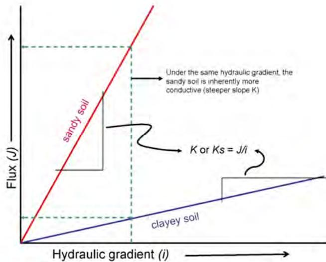
**Figure 6-3 Relationship between specific discharge and hydraulic gradient**
