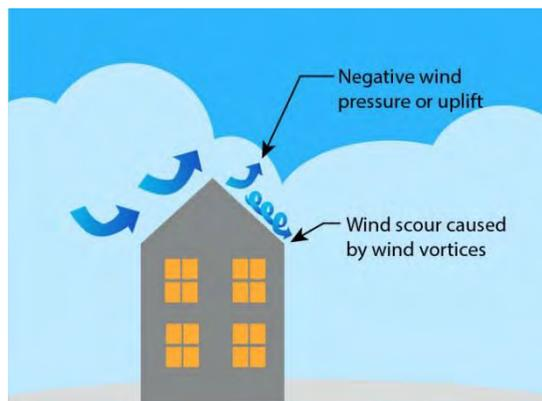
*Figure 12-9 Effects of wind on roofs*
