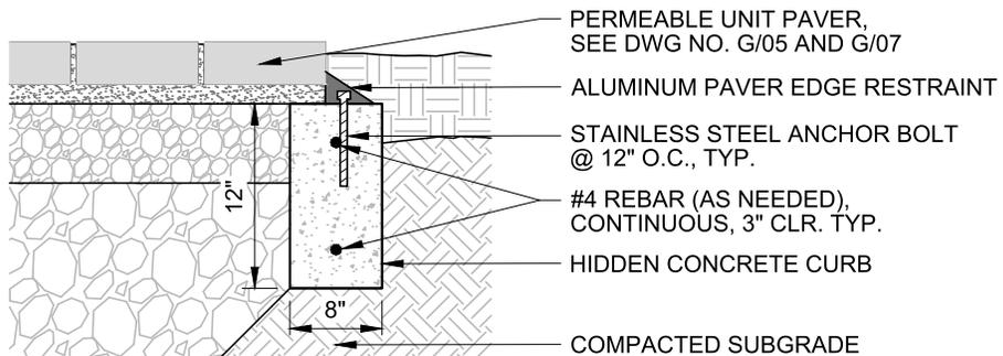
**METAL EDGE RESTRAINT ON HIDDEN CONCRETE CURB
