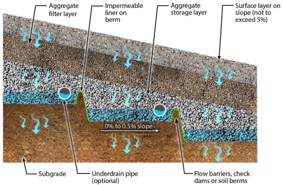
**Figure 10-20 Steep slope drainage profile with subgrade terraces**
