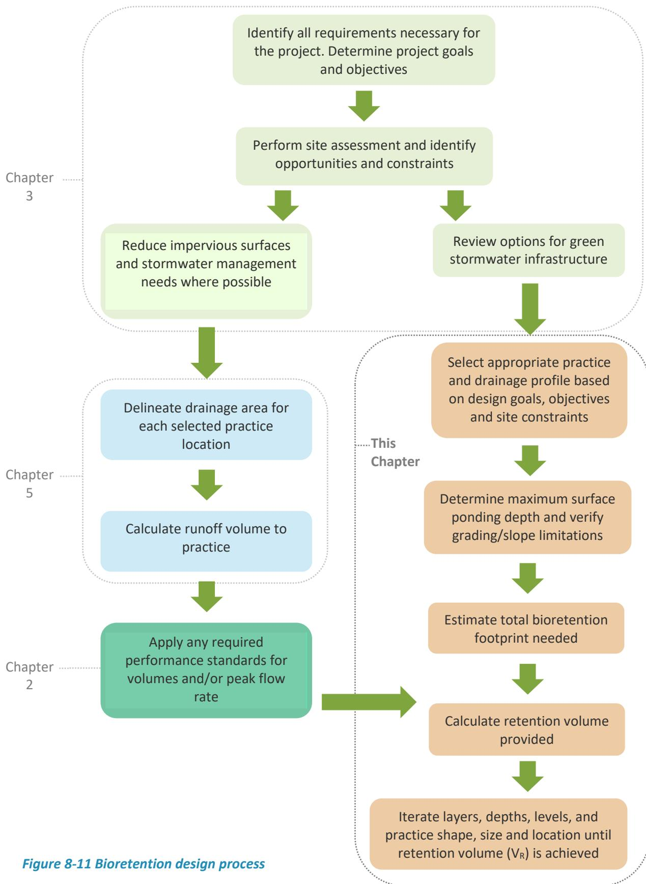
Figure 8-11 Bioretention design process
