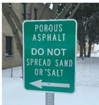
*Figure 10-35 Signage to remind maintenance staff of the presence of permeable pavement*
