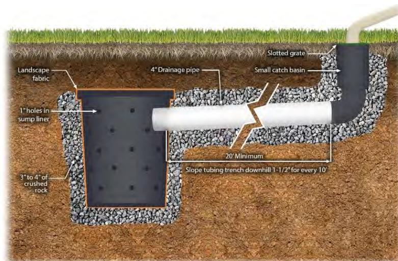
Figure 9-7 Dry well attached to roof downspout
