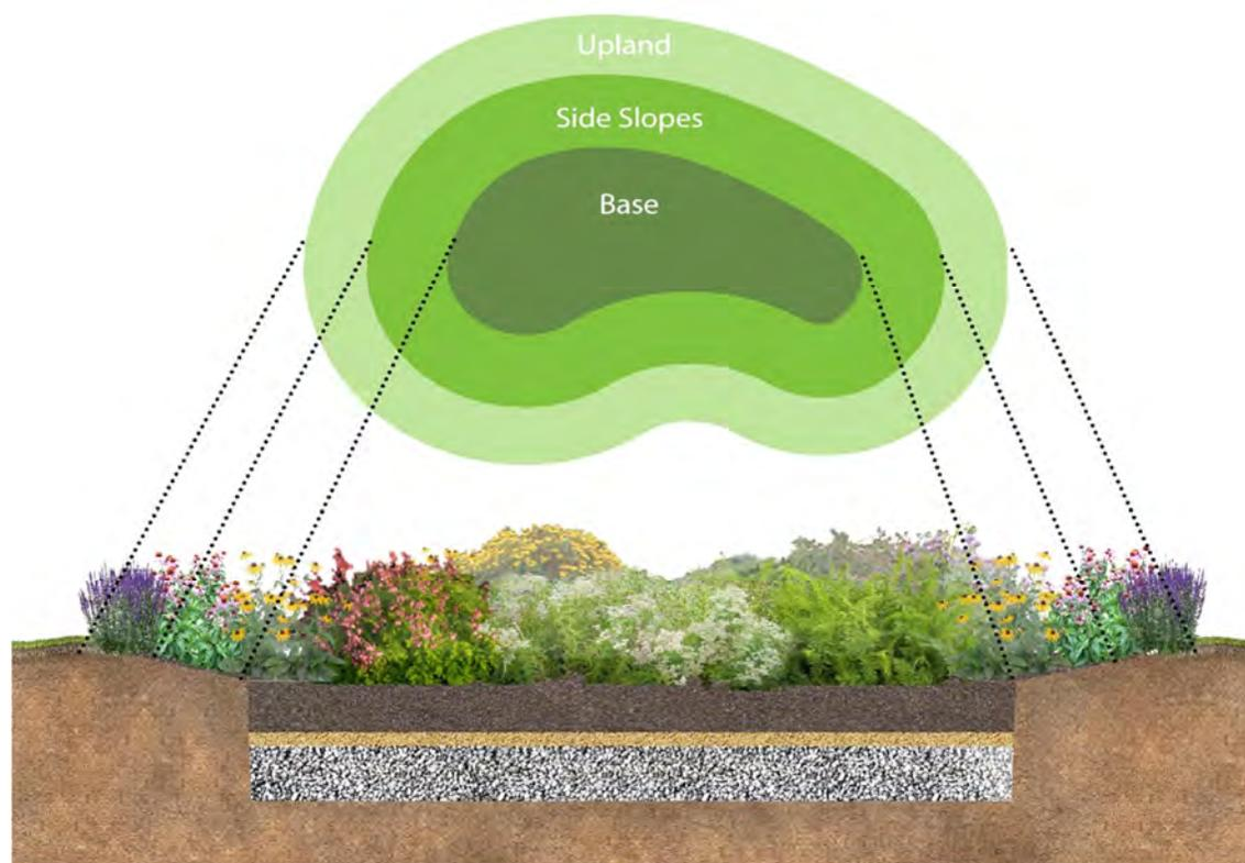
*Figure 8-35 Hydrologic Zones of a Typical Vegetated GSI Practice*
