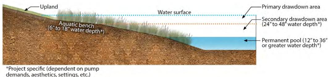
**Figure 7-12 Hydraulic Profile of Detention Practice for Reuse**
