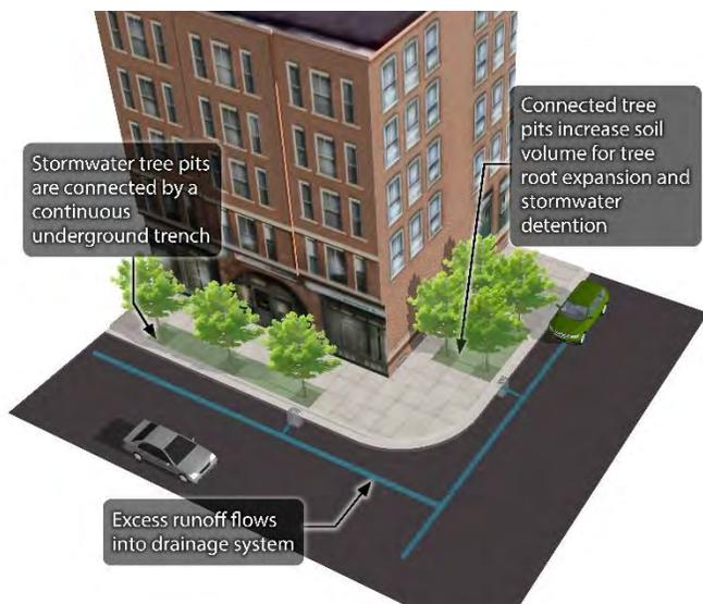
Figure 15-6 Interconnected tree pits
