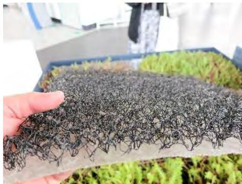
*Figure 12-10 Living roof drainage layer*
