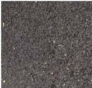
**Figure 10-3 Example of Porous Asphalt**
