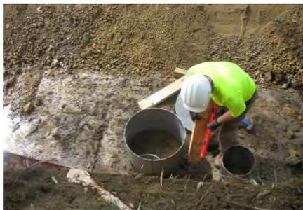
**Figure 1-2 Soil infiltration test**
