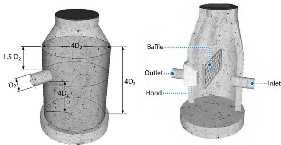
**Figure 5-8 Inlet Structure with Sediment Sump**
