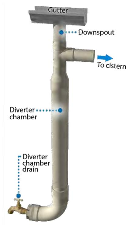
Figure 11-6 First-Flush Diverter
