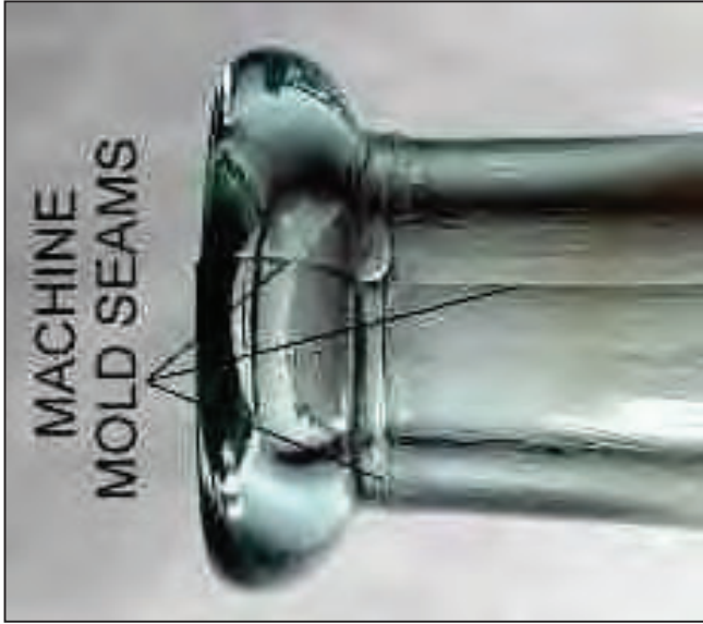
Mold Seam on and over Bottle Lip
