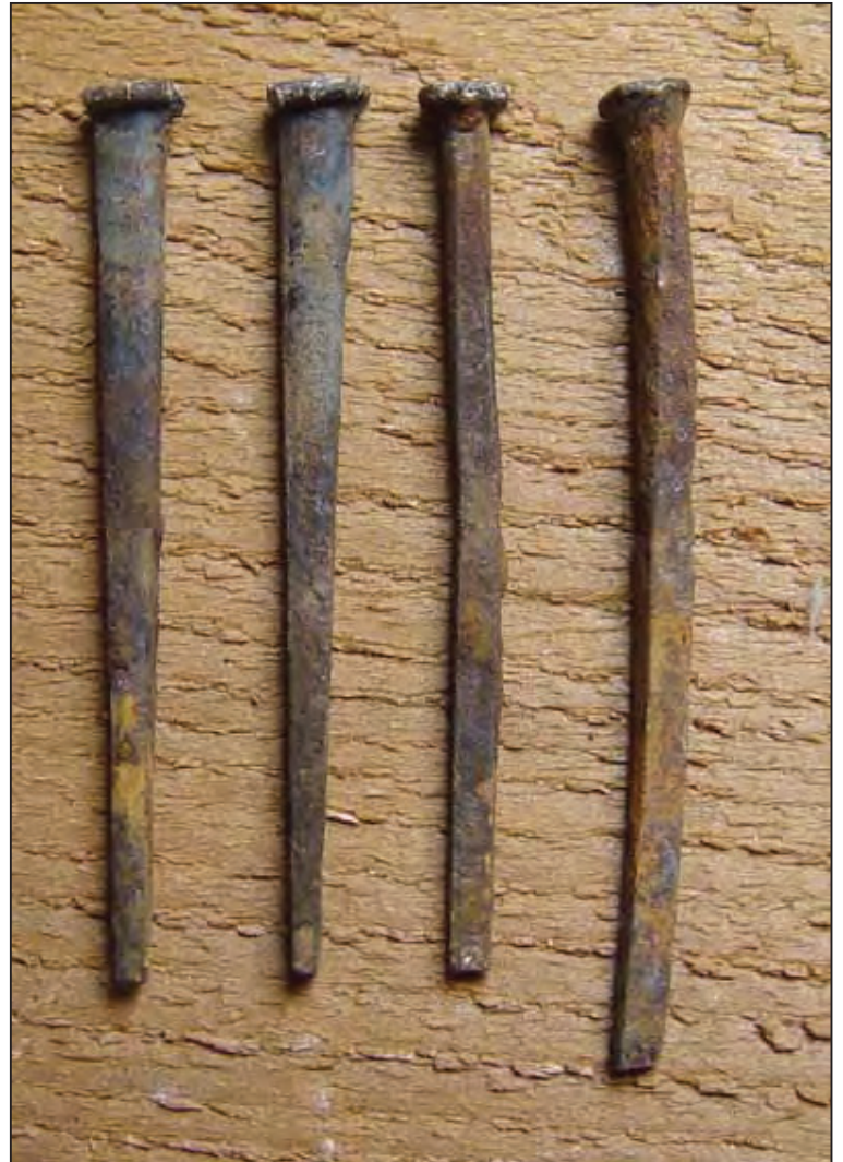
Machine-cut Square Nails (ca. 1805-1890)
