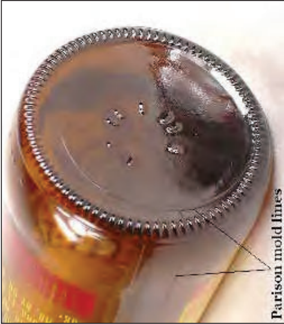
Mold Seams on Machine-made Bottle
