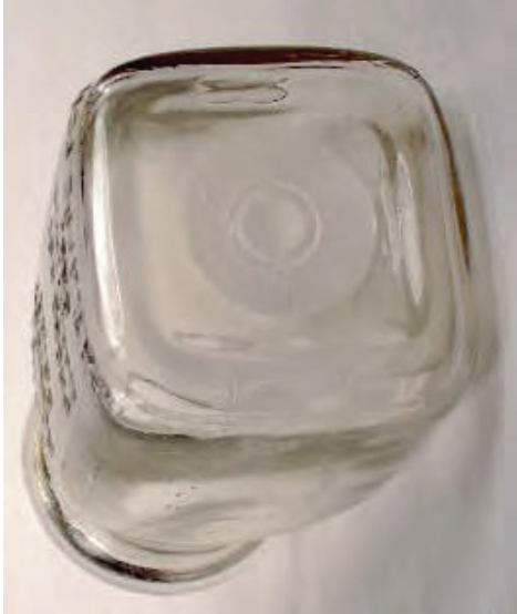
Valve Ejection Mark on Dairy Bottle Base
