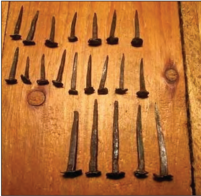
Hand-forged Nails (prior to 1820)
