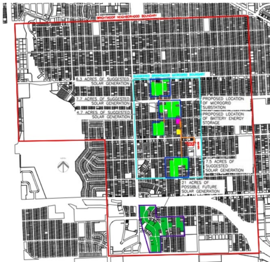
Fig. 3. Proposed layout for Brightmoor neighborhood microgrid.
