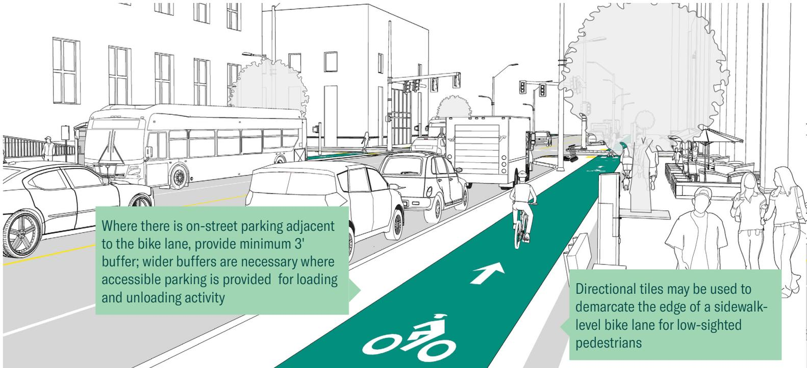
Where there is on-street parking adjacent to the bike lane, provide minimum 3' buffer; wider buffers are necessary where accessible parking is provided for loading and unloading activity
