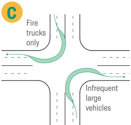
Accomodate turns with recessed stop bars and signal phasing at signalized intersections
