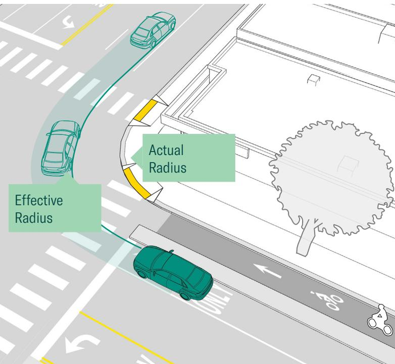
**Actual radius** involves the curve that the face of the curb line makes at the corner. **Effective radius** refers to the real curve created by motor vehicles in turning and is enlarged from the actual radius by the presence of on-street parking, bike lanes, and other features.
