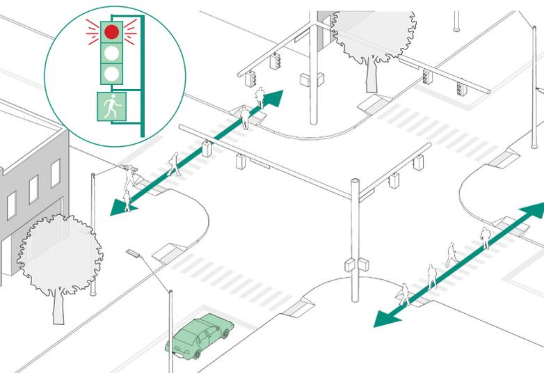
Pedestrians given walk signal to enter crosswalk ahead of waiting driver to increase visibility and reduce delay
