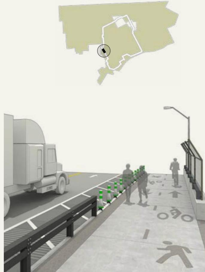
Dimensional constraints limit path width in this section. The proposed configuration allows adequate space for large trucks to maneuver while keeping greenway users safe. Rumble strips adjacent to the cycle track warn drivers of their proximity to the edge of the roadway, further enhancing user safety.
