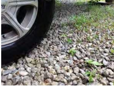
Figure 10-7 Example of Open Graded Aggregate as a Pavement Surface
