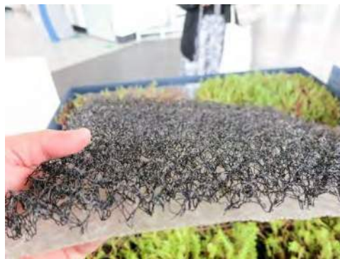
Figure 12-10 Living roof drainage layer
