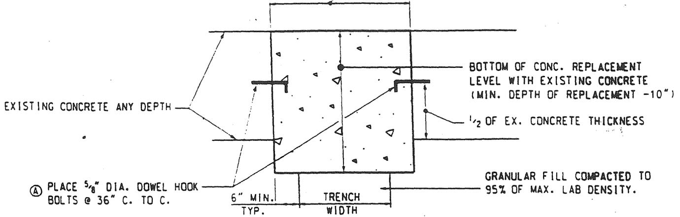
1. REPLACEMENT WIDTH IS DETERMINED BY TRENCH LOCATION WITH RELATION TO LONGITUDINAL JOINTS. SEE SHEET NO. 4.
