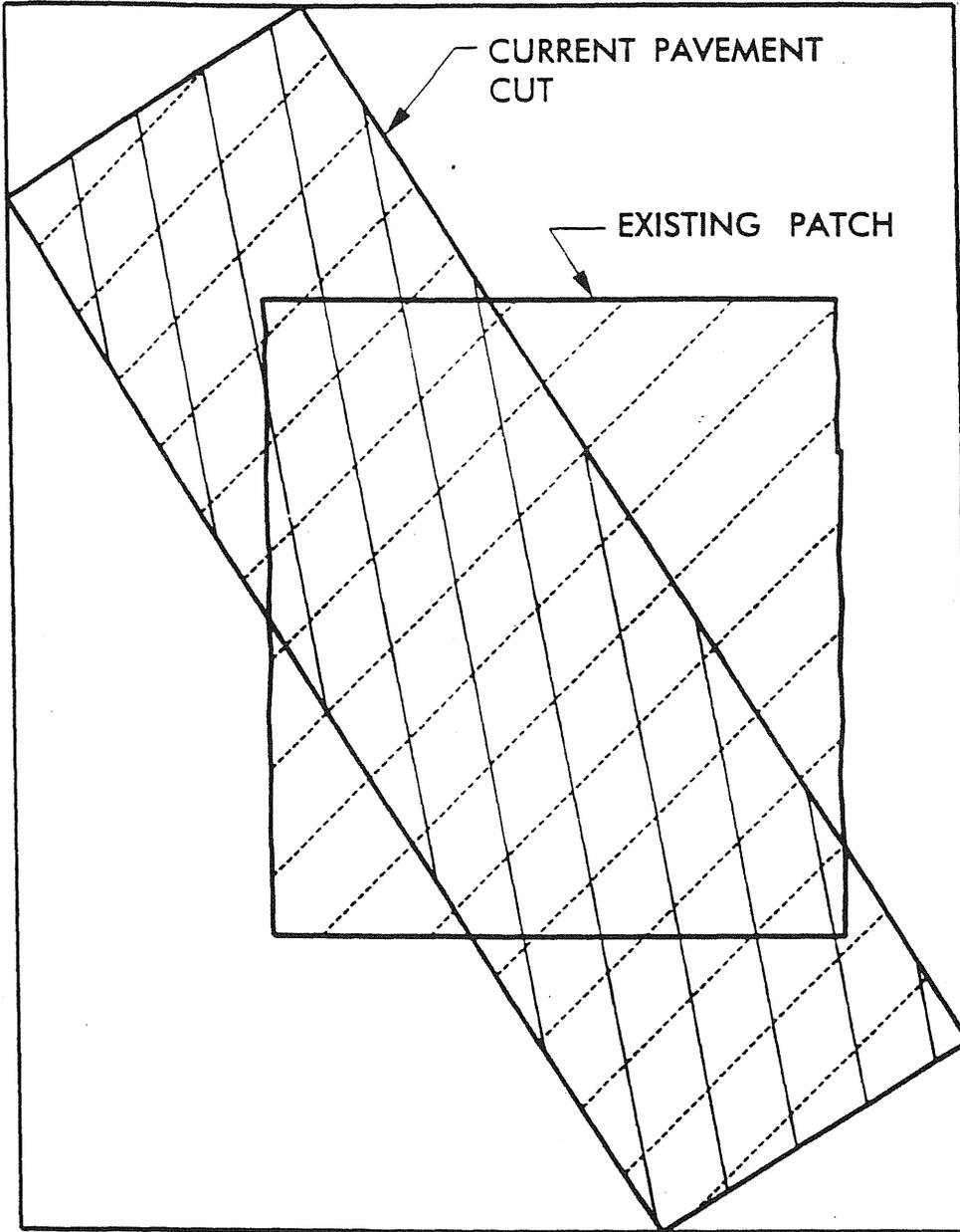
LIMITS OF CONCRETE OR ASPHALTIC BASE AND SURFACE REPLACEMENT IN CONCRETE PAVEMENTS, IF THIS LINE IS CLOSER THAN 3 FEET FROM THE ADJACENT JOINT LINE, THEN THE PAVEMENT SHOULD BE REPLACED TO THAT JOINT.
