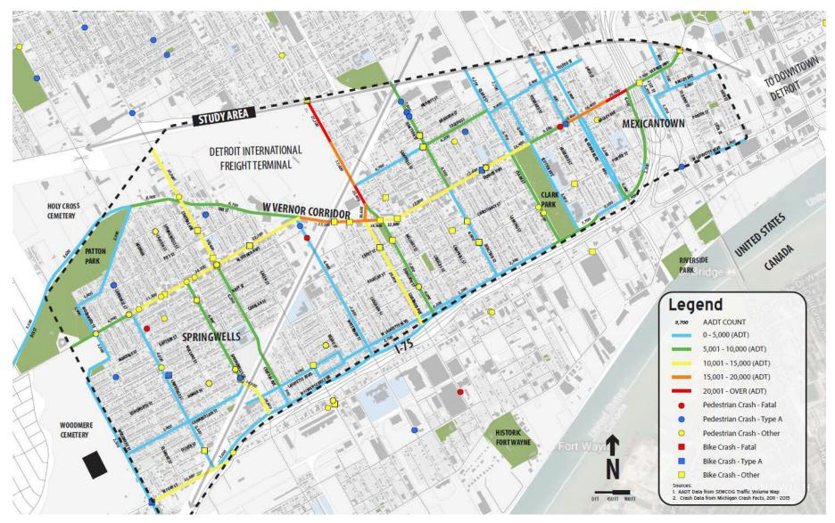
The study area contains a number of busy streets, but traffic levels along most segments are in a range where simple, proven elements like crosswalk bump-outs, protected bike lanes, and street trees can significantly improve the safety and appeal of walking and biking.
