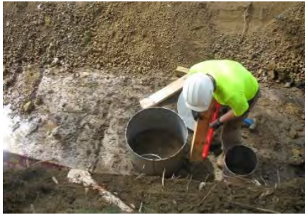
Figure 1-2 Soil infiltration test
