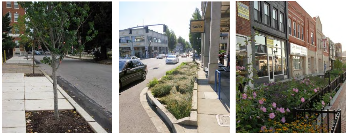
Figure 3-11 Three examples of green stormwater infrastructure practices in commercial district with similar benefits but different designs and costs. From left to right: tree based suspended pavement (Philadelphia PA), curb extension bioretention (Portland OR), and planter box (Lansing, MI)
