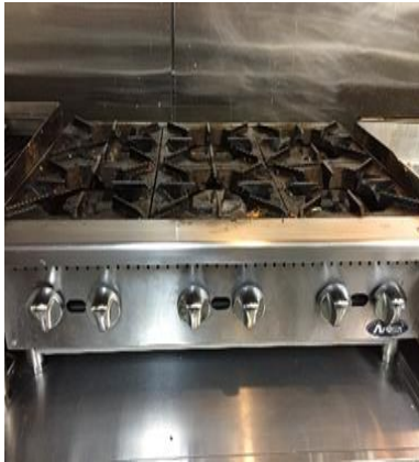
Counter top equipment elevated on 4-inch legs to provide space for cleaning underneath
