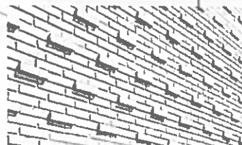
BRICK White with relief pattern @ fascia band
