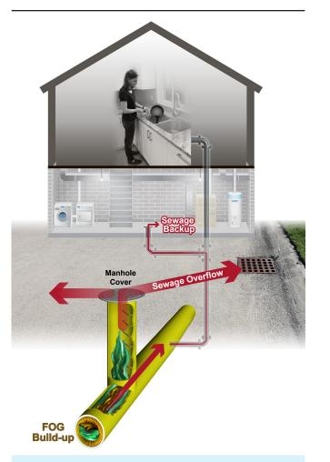
Before reaching its ultimate destination of GLWA's WRRF in Detroit, sewage flows through a network of pipes that are operated by different entities.
