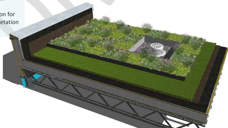
Figure 12-1 Typical living roof
