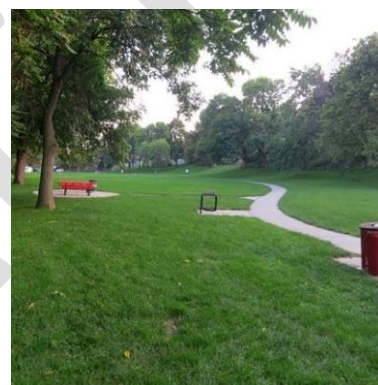
Disconnected impervious sidewalk draining onto lawn
