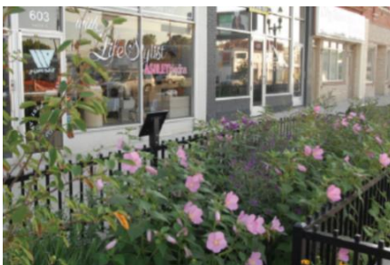
Bioretention between road and sidewalk
