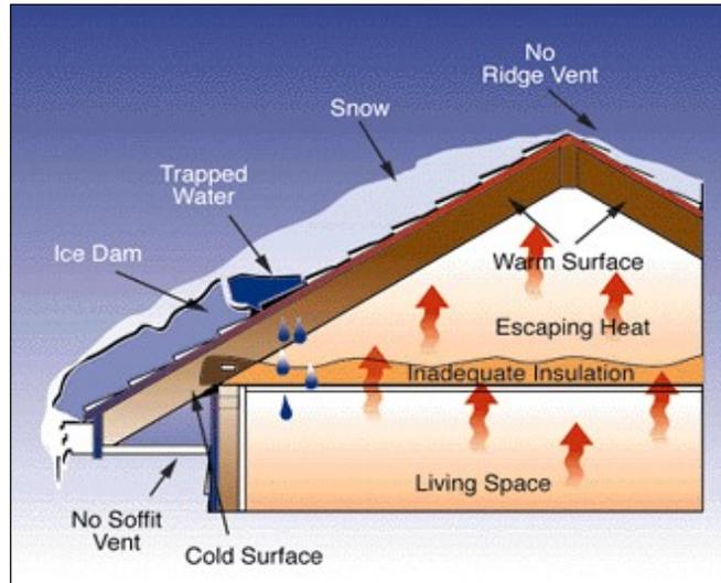
Roof ice dams occur in climates with freezing temperatures and significant snowfall. When the temperature in the attic is above freezing, snow on the roof melts and runs down the sloping roof. When the snowmelt runs down the roof and reaches the colder eaves (overhang) and gutters, it refreezes.
