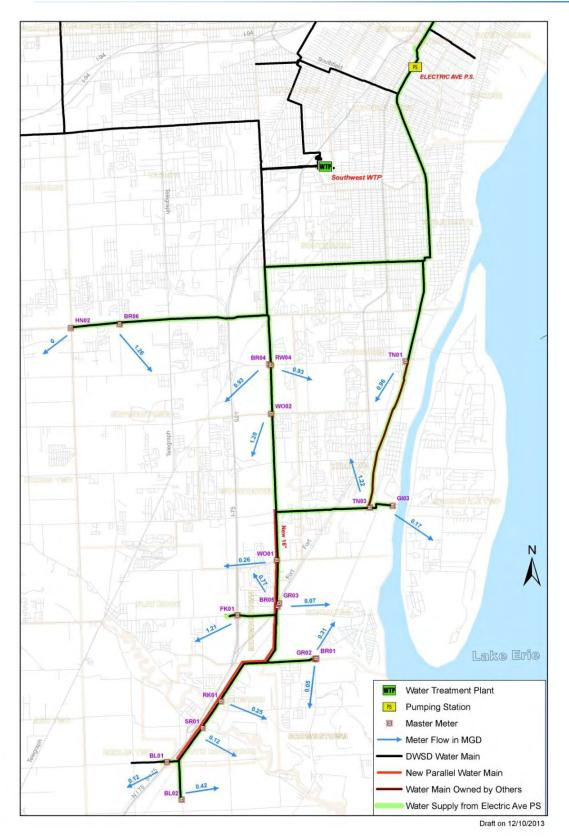
Figure 7-6: Alternative 4 – Supply from Electric Ave PS and Parallel Pipeline along Allen Rd./Dixie Hwy
