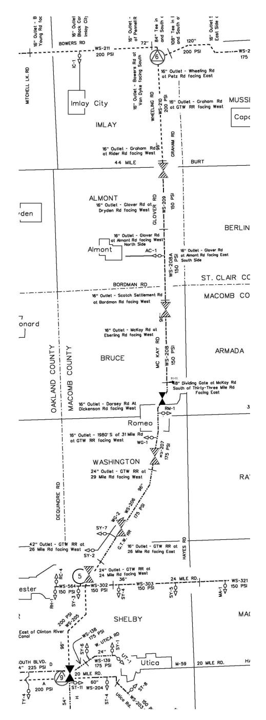
Figure 7-16: Proposed Isolation Valves for 96-Inch Transmission Main
