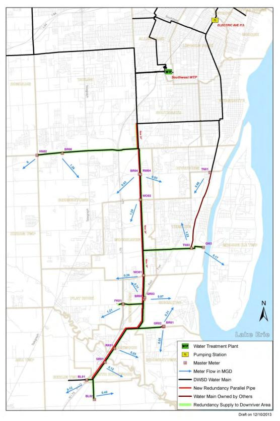
Figure 7-4: Alternative 2 – Parallel Pipeline along Allen Road/Dixie Hwy
