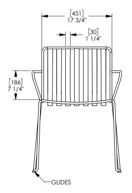
Drawing: DX101-02 Dimensions are in inches [mm]
