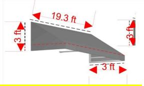
Awnings to be Mounted to Inside and Window Frame 8ft height is allowed from Grade to Top of Awning Area
