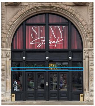
Approximate dimensions of proposed awning, stated to be 18' wide and 8' from grade. Illustration by staff based on field measurements.
