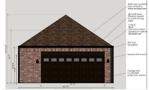
Figure 1, by Applicant: Proposed front elevation of garage showing pyramid roof, brick cladding, wood trim, wood doors.
