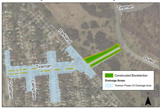
Figure 10: Tireman Bioswales - Drainage Areas
