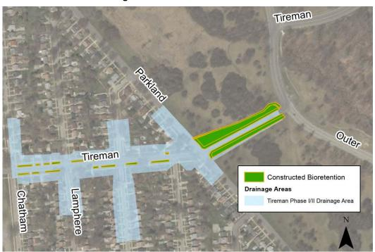
Figure 10 Tireman Bioswales - Drainage Areas
