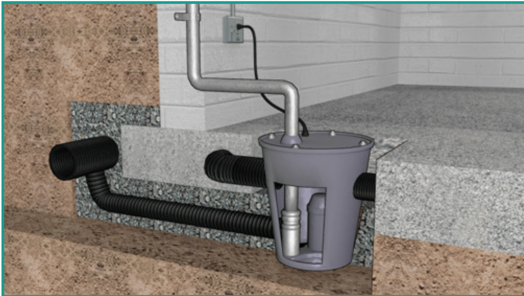
A sump pump attached to the drain tiles around a basement foundation
