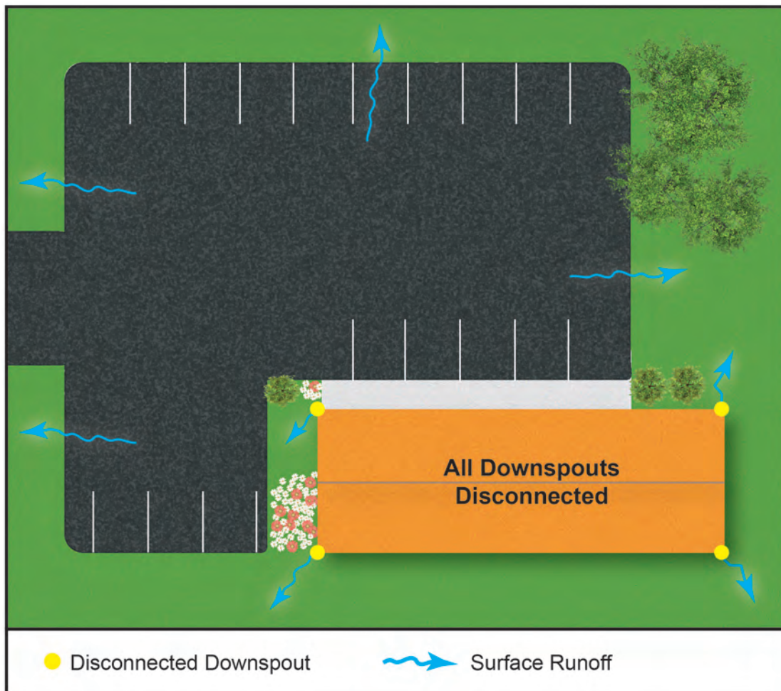
Figure 11: Disconnected Downspouts Draining to Pervious Area
