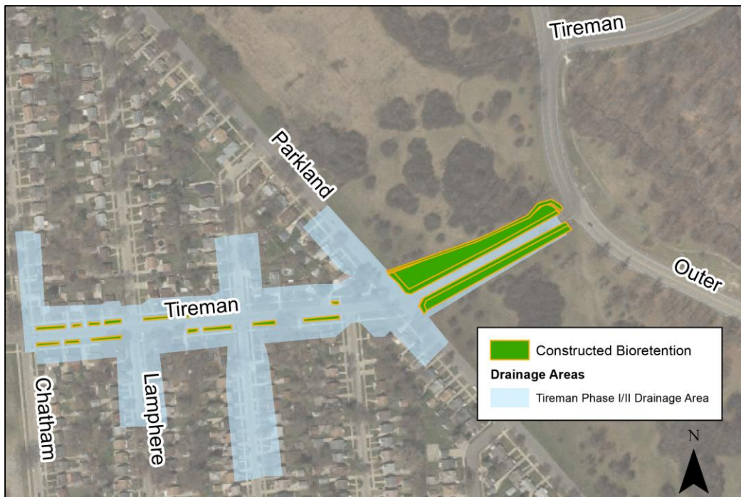
Figure 10 Tireman Bioswales – Drainage Areas
