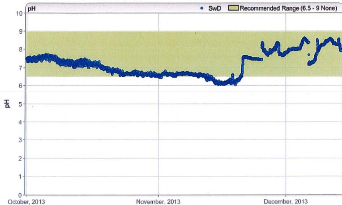
Figure 2-24: Southwest WTP pH
